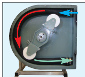
Each 180° the opposite rollers compress the hose in two places and the motion is continued.
